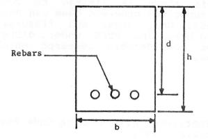
Figure 1. A Simply Supported Reinforced Concrete Beam
