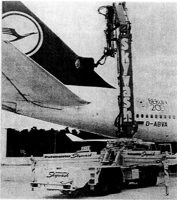
Figure 1: Washing robot at the Aircraft
