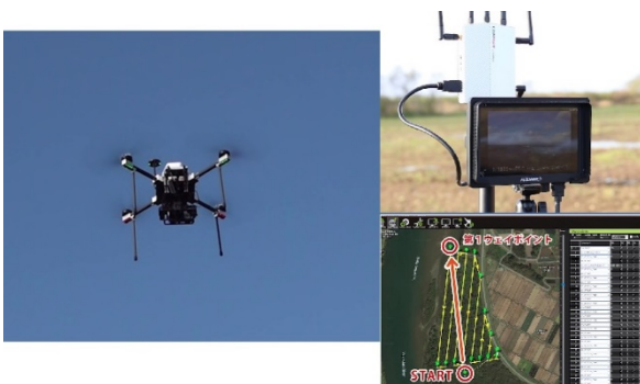
Figure 4. The UAV surveying (UAV, monitor, flight control system)
