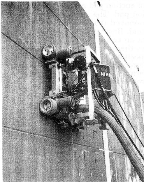
Photograph 1 Robot travelling along a wall surface
