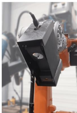
Figure 2. Keyence LJ-X8400 Line Profiler Head attachment to the flange of KUKA KR30-3 F Robot arm
