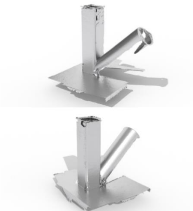
Figure 8. Constructed mesh preview with 6 scans, total computation time 8 minutes at robot speed of 3mm/sec.
