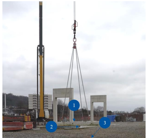
Figure 7. 1) Component weight ~1000 kg 2) Distance sensor, which measures the distance to the floor, to record the oscillation
