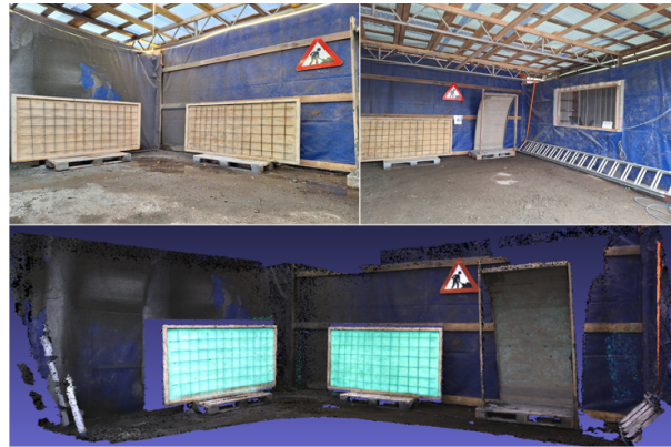
Figure 4. Upper part: samples of two images of the testing area within the construction site. Lower part: semantically annotated 3D mesh model, where regions of interest are highlighted in cyan.
