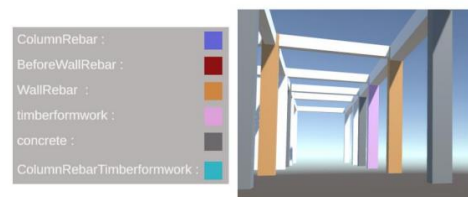
Figure 7. Query and display different colors corresponding to the construction phase
