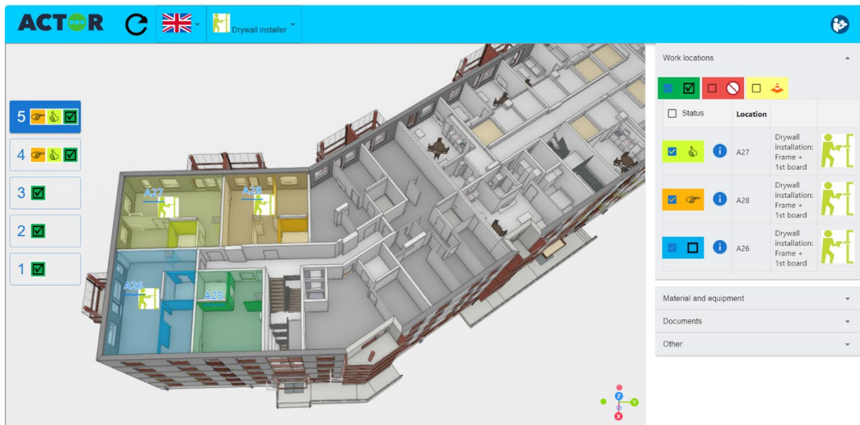
Figure 2. DVM Info screen View for a Selected Floor with Visualization of Work Status of Drywall Installer
