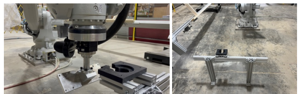
Figure 4. The tool stand and pneumatic tool changing system
