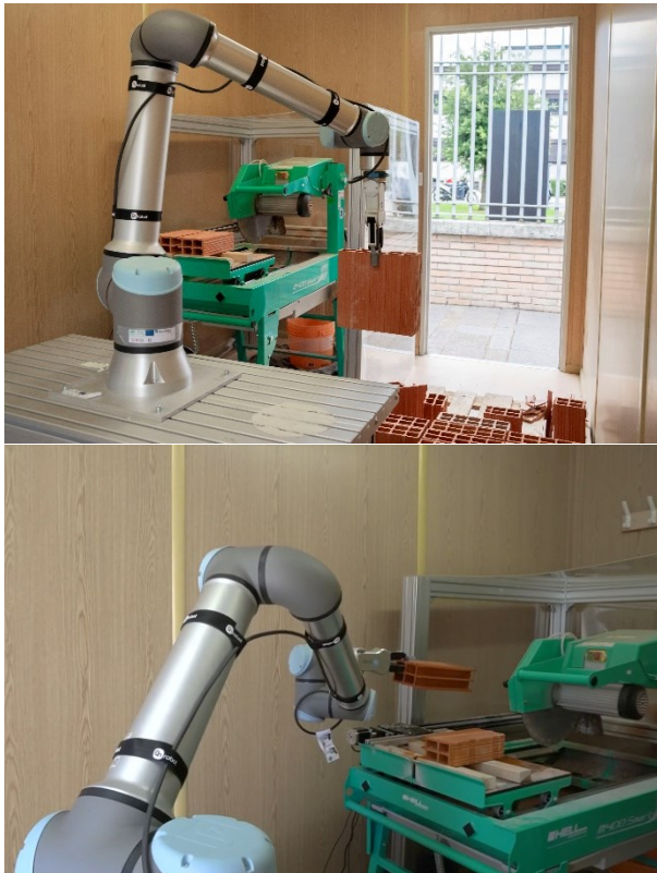
Figure 7 a/b: Automated brick cutting system
