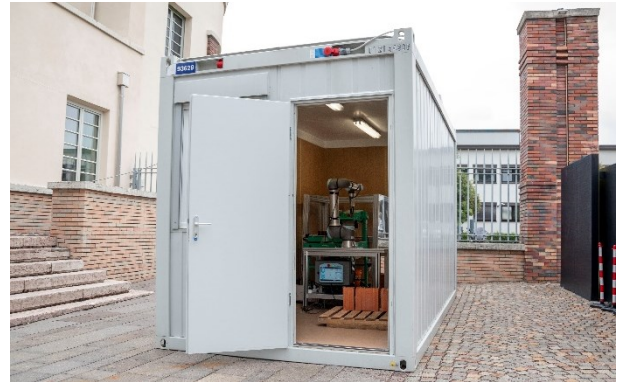
Figure 6. The construction container - Automated on-site prefabrication
