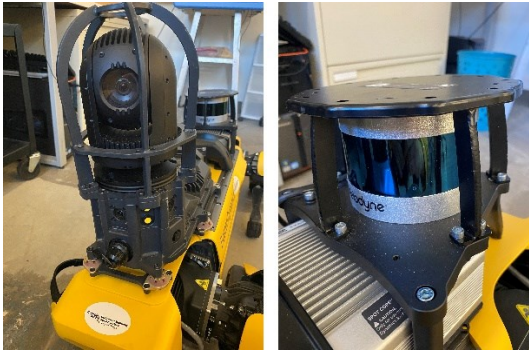
Figure 4. Spot CAM+ payload, and spot Core I/O and Velodyne VLP-16 LiDAR
