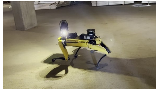
Figure 2. Boston Dynamic's SPOT with 360° camera and a LiDAR payload.
