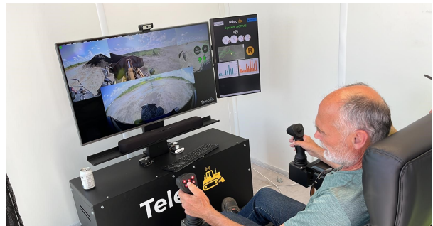
Figure 4. Control booth of retrofit remote control system.[22]
