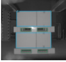
Figure 11 Pallet and material detection
