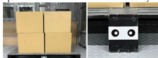
Figure 9 Skid pallet marker
