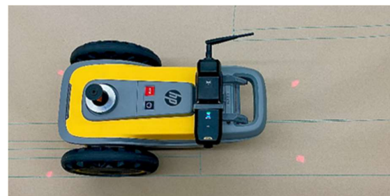
Figure 3. HPSitePrint Safety Sensors
