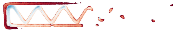
Figure 10. Height deviation map of the 21st layer (the last layer) shortly after the printing process.
