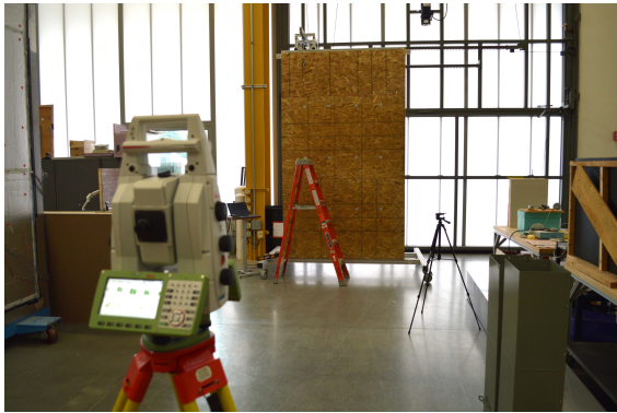
Figure 6. Setup of the connection locating system experiment.
