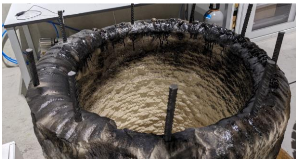
Figure 8. Printed and coloured PU-foam column for evaluation. The rebar was added to the last layer and the camera was moved along the printing trajectory over the surface for one full circle. Movement speed was set to 100mm/min
