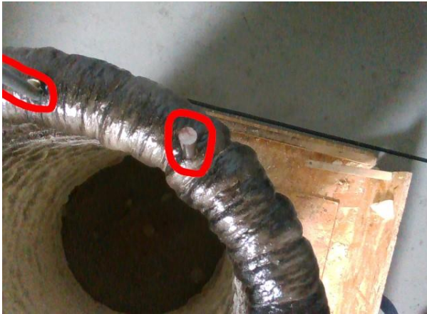
Figure 4. 3D printed PU-foam strand with inserted short reinforcement bars marked by red circles.
